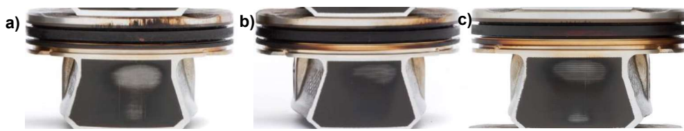
Figure 2.2. Land cleanliness differences between a) in Group II base oil b) in Group II base oil with extra dispersant c) in Group III base oil environments.
